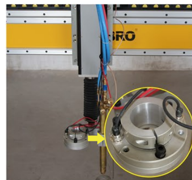
Anti-collision THC protect the torch
